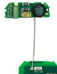
X24-SAe ATEX/IECEx Telemetry Strain Transmitter OEM Module
